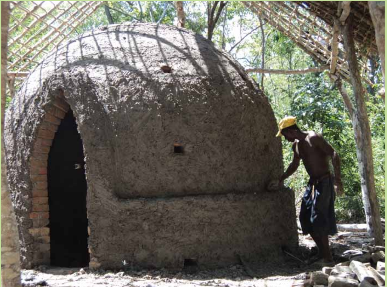
The Half Orange Kiln, which recovers up to 45% with 3-4 days of work
