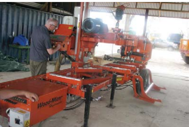
Bioshape saw mill for processing timber from coastal forests on their farm
