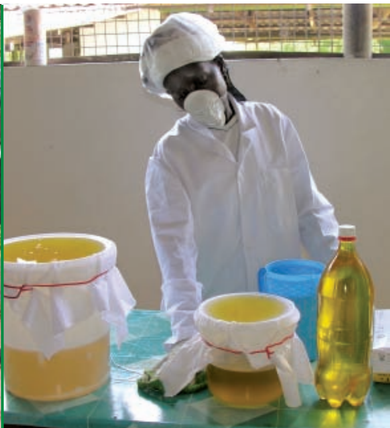
A member of the community from the neem-based Salama Hewevu Bio-enterprise in Tana River filtering extracted neem oil Photo by ICIPE
